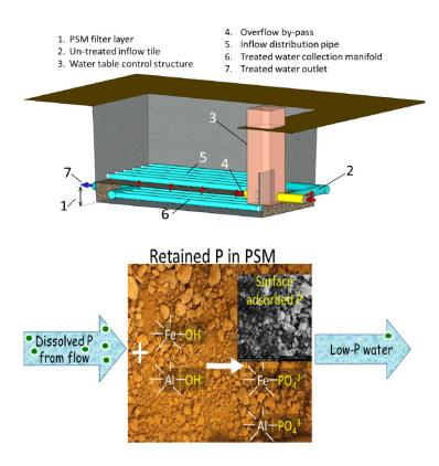
Example of a P removal structure and components, specifically a subsurface tile drain P filter using iron and alumunimum metal hydroxides.
