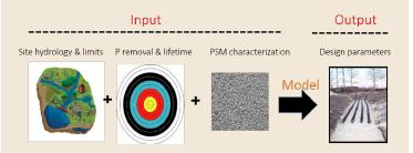
Structures are constructed based on a desired P removal goal and lifetime in accordance with site conditions (flow rate and DP concentration). For example, a 10yr-40% goal means that the structure is designed for removing 40% of all the DP that flows into a structure over 10 years. For details on P removal structures and how to gather inputs, see <u>Penn, C.J., and J.M. Bowen. 2017. Design and construction of P</u> removal structures for improving water quality. Springer Publishing.
