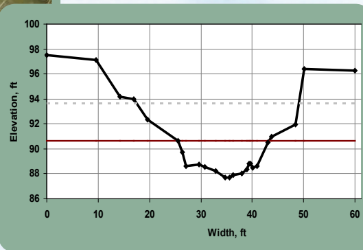
Figure 6. Deeply incised ditch with extensive scour and slumping on outer bends but some point bar (bench) formation on the inner bends (above); the representation of this measured cross-section in the Reference Reach spreadsheet tool (right).
