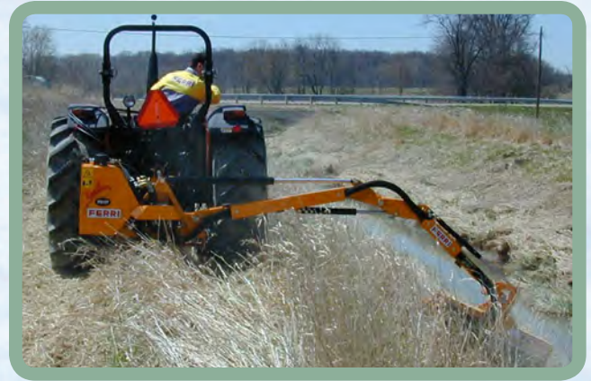
Figure 2. Mowing an agricultural drainage channel. (source: http://www.ferri-america.com/boom-mowers )
